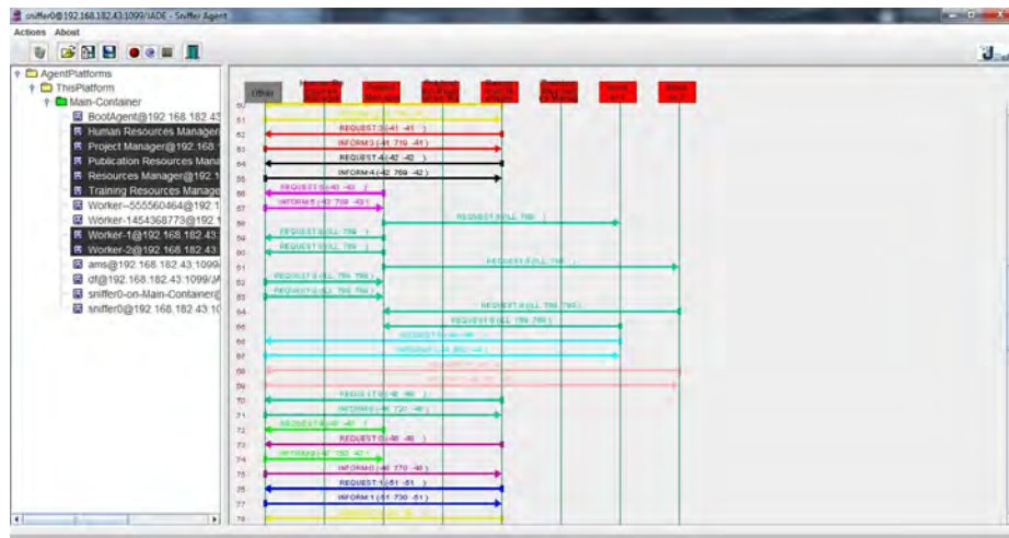
Fig. 14. Communication process—messages sent in the system—captured by JADE Sniffer Agent
