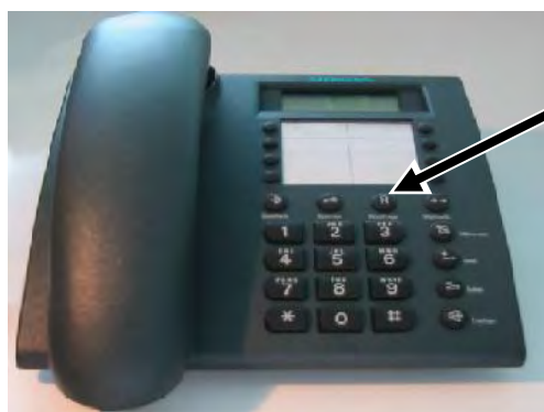
Fig. 2. Standard telephone interface with a flash-hook button (labeled with "R")
