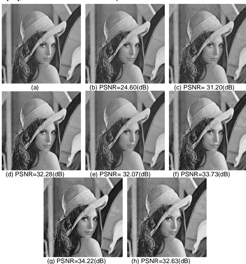
Fig.5. (a) original Lena image; (b) noisy image: N(0,15) ; (c) Y-K [27], Time=152.04(s); (d) LLT [28], Time=10.20(s); (e) non-local mean [4]; (f) LARK [2], Time=570.09(s); (g) BM3D [8], Time=6.99(s); (h) proposed GVC-based Y-K, Time=120.27(s).
