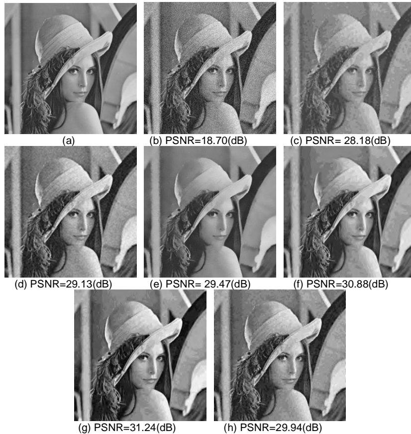
Fig.6. (a) original Lena image; (b) noisy image: N(0,30) ; (c) Y-K [27], Time=654.21(s); (d) LLT [28], Time=26.73(s); (e) non-local mean [4]; (f) LARK [2], Time=1419.20(s); (g) BM3D[8], Time=7.04s; (h) proposed GVC-based Y-K, Time=450.28s.
