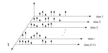
Fig.3. The impulse response of the time-varying channel
