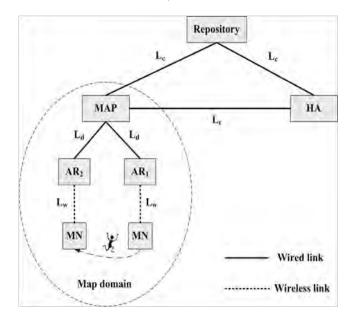
Fig.6. System model for transport latency analysis
