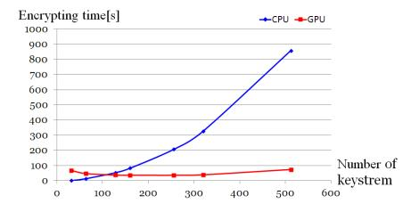
Fig. 5. Comparison of encryption time between CPU and GPU.
