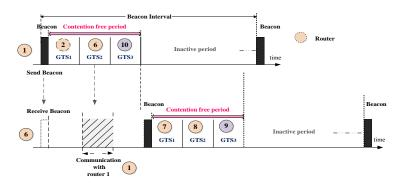
Fig. 3 The relation between router and child device
