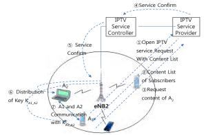
Fig. 8. Pairwise key establishment between devices for open IPTV in the same cell
