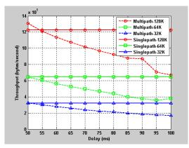
Fig. 15 Multipath vs Single path (adjust RTT in one path) for Scenario three
