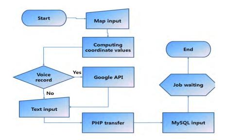
Fig. 11. A flowhchart for inserting coordinate values
