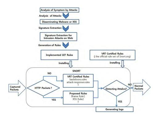
Fig. 4. Process of signature-based detection
