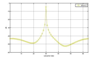
Fig. 8. The ICI power for the desired signal at subcarrier 30
