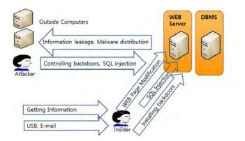
Fig. 2. Intrusion Path of Detoured Attacks
