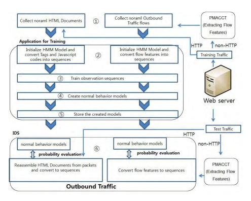
Fig. 5. Process of anomaly-based detection
