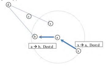
Fig. 3. Location-based routing protocol
