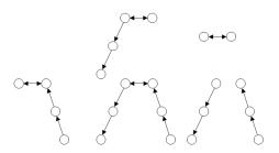
**Fig 3.** The Valley-free Path in BGP Policy. A valley-free path is a path has zero or several customer-provider sequences followed by one or zero peer-peer edge and then followed by zero or several provider-customer sequences.
