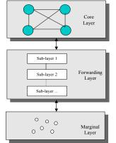
**Fig. 1.** Three Tiers Model Literature of Internet. a)The set of nodes who have no providers forms a clique is the core layer.b) If the nodes don't forward data for others, then it belongs to the marginal layer.c) The node that belongs to neither the core layer nor the marginal layer belongs to the forwarding layer.
