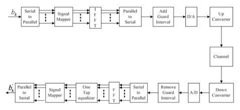
Fig. 1. Block diagram of OFDM systems
