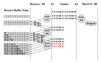
Fig. 3. Receive buffer blocking caused by packets loss
