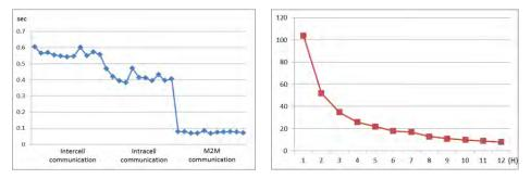
**Fig. 11.** Communication and rekeying overhead (a) Time for communication between devices as a function of distance (b) Number of packets as a function of group key rekeying frequency in 24 hours.
