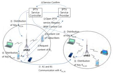
Fig. 9. Pairwise key establishment between devices for open IPTV in different cells
