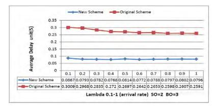
Fig. 6 Packet average transmission delay (SO=2 BO =3)
