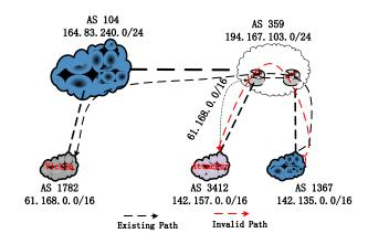
**Fig 2.** AS 3412 hijacks the prefix of AS 1782. AS 3412 has the IP prefix of 142.157.0.0/16 and AS 1782 has the IP prefix of 61.168.0.0/16. But AS 3412 in order to hijack the flow of AS 1782, it announces a BGP Update that it has the IP prefix 61.168.0.0/16. AS 1367 changes its path to the destination prefix 61.168.0.0/16, and its data to AS 1782 would be transmitted to AS 3412.
