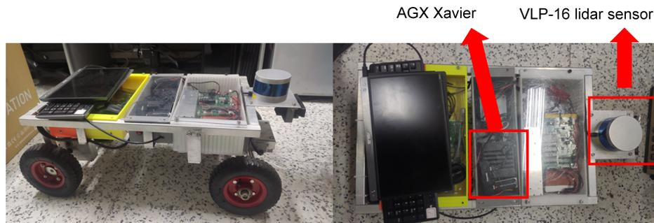
**Fig. 2.** Designed autonomous Ackerman robot
