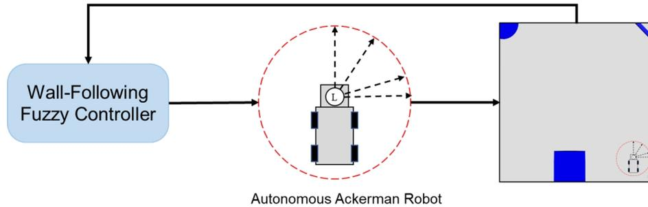
Fig. 5. System flow of the wall-following mode
