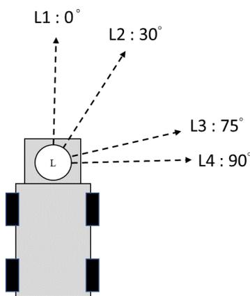
**Fig. 9.** Four directions sensed by the lidarsensor
