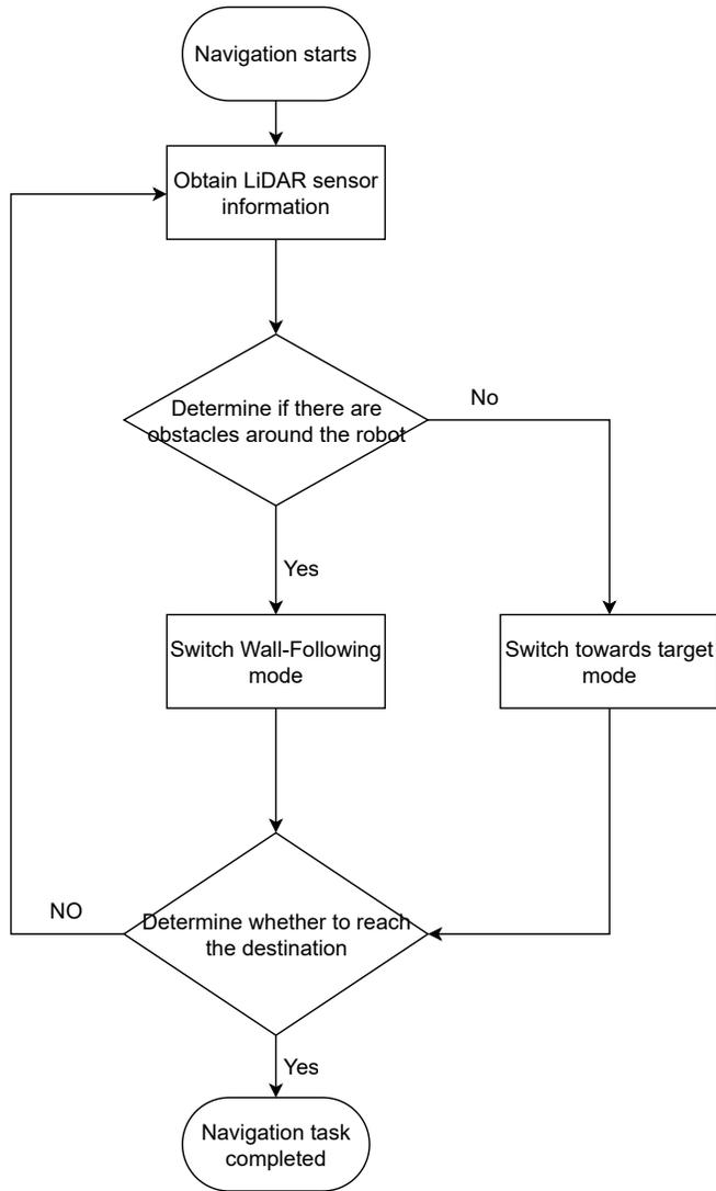
**Fig. 1.** Flowchart of the proposed navigation system
