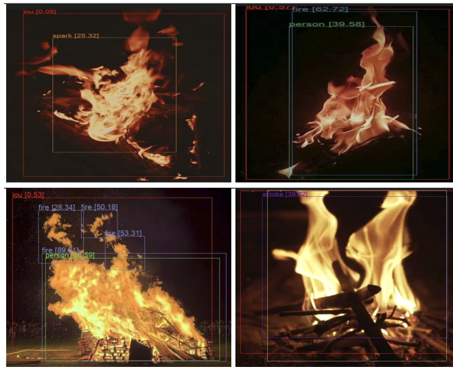
Fig. 10. Red color B/B indicates ROI, Top Left (TL) image is incorrectly recognized as a spark, Top Right (TR) image is incorrectly recognized as Fire and Person, and Bottom Left (BL) image is Fire and Person. In the case of Bottom Right (BR) images, it is mistakenly recognized as smoke
