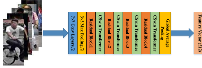
Fig. 5. The main architecture of the combination of Residual Block and Swin Transformer for feature learning.
