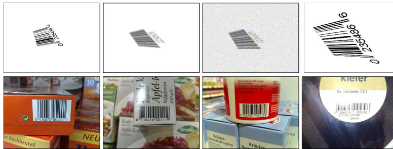
Fig. 9. 1D samples with different distortions, synthetic (first row) and real images (second row).
