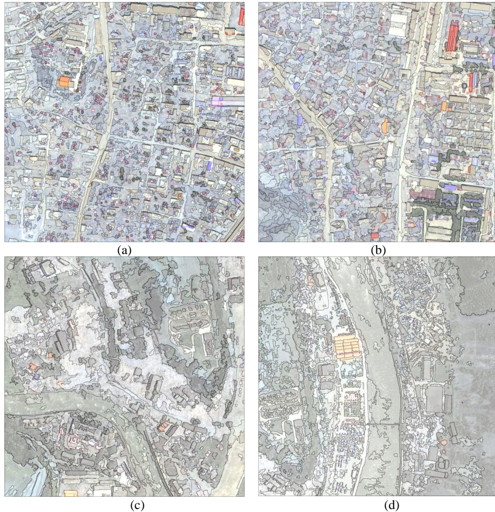
Fig. 3. WJSEG segmentation and initial object set extraction results: (a) Dataset 1; (b) Dataset 2; (c) Dataset 3; (d) Dataset 4.
