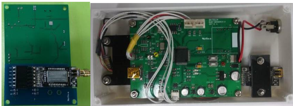
Fig. 9. The sensor board with an LPWA communication module applied, and the inside of the PM sensor module
