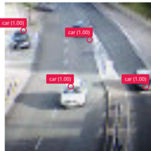
Fig. 7. Object detection from Arduino camera shown in browser
