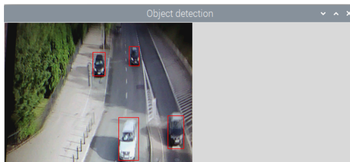
Fig. 8. Detection of vehicles using DL models deployed on RPi
