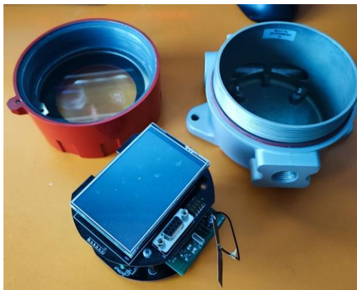
Figure 1 Developed IoT node before sealing in the safety Ex e casing
