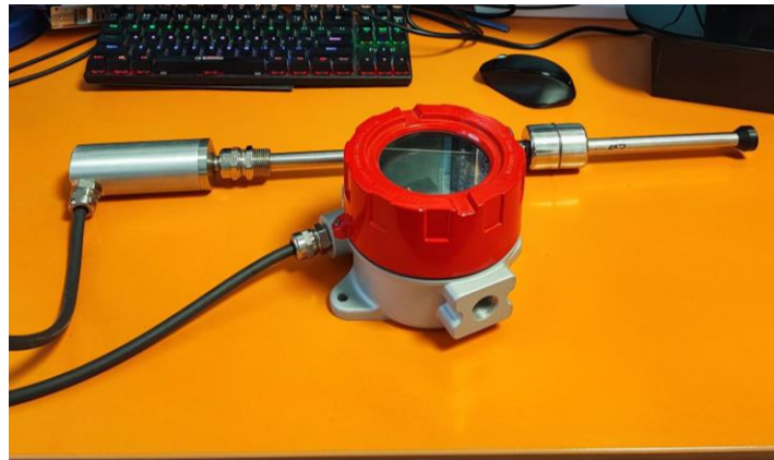
Figure 11 Finalized IoT node with one RS485-based sensor attached
