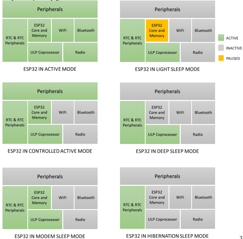
Figure 4 Comparison of active elements in ESP32 standard working modes and Controlled Active Mode
