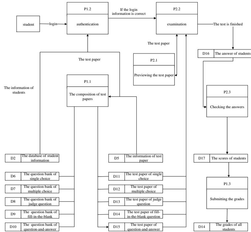
Fig. 4. The detailed flow chart for student and server
