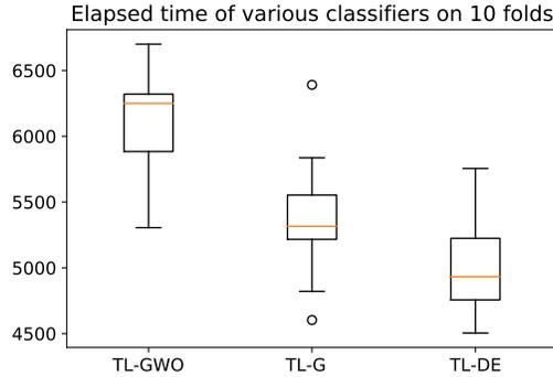
**Fig. 5.** Comparison of consumed time for training for the three HPO-TL methods.
