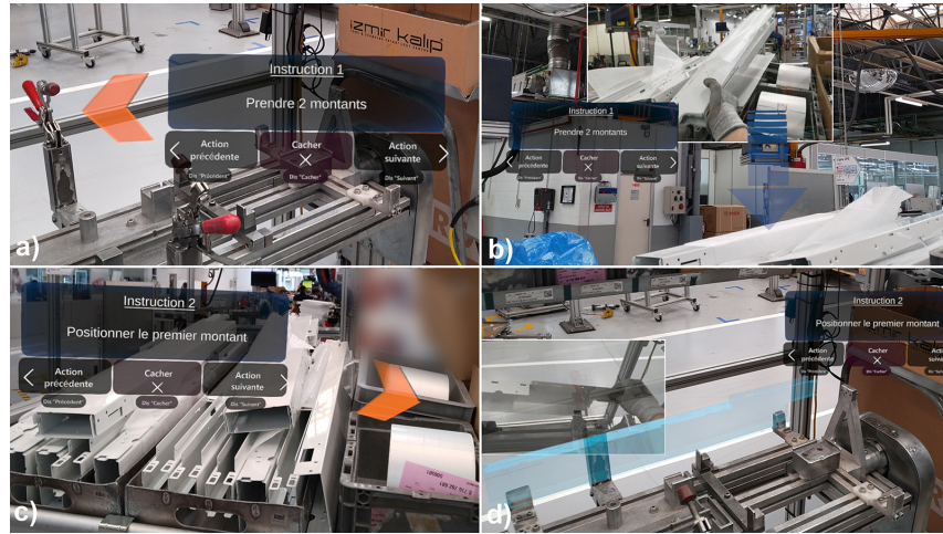
Fig. 2. AR training example: a) Instruction 1a: text description (“grab 2 uprights”) & directional arrow; b) Instruction 1b: Location arrow & FPV image illustrating the operation; c) Instruction 2a: text description (“place the 1st upright”) & directional arrow; d) Instruction 2b: Location arrow & FPV video demonstrating the assembly operation.
