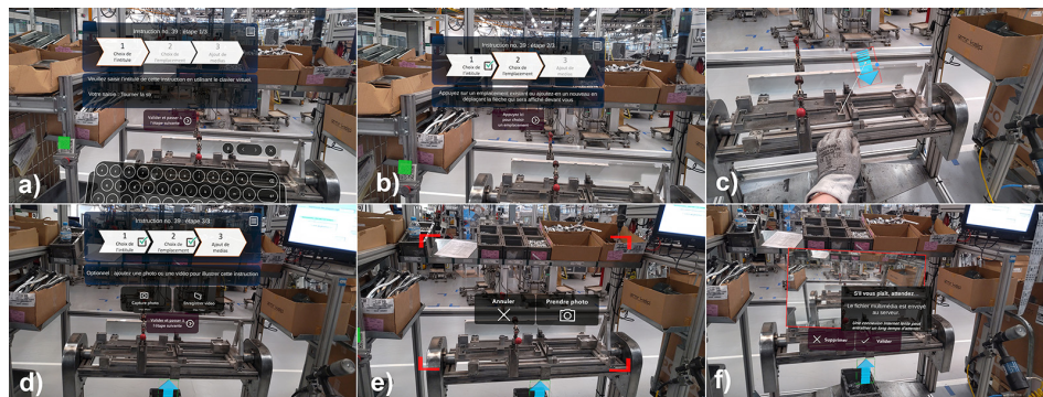
Fig. 1. AR authoring example. a) Step 1. Insert text instruction by using the virtual keyboard or dictation; b) Step 1 validated, step 2 active; c) Step 2. Positioning of the location arrow by using far interaction technique; d) Step 2 validated, step 3 active; e) Step 3. Photo-capture view; f) Step 3. Photo taken, the author validates or removes it.
