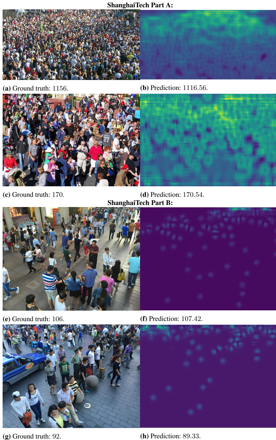
Fig. 4. Images in the left column represent input images from the ShanghaiTech part A (a – d) and ShanghaiTech part B (e – h) test sets, with 1156, 170, 106, and 92 annotated people, respectively. Images in the right column represent the predicted density maps obtained by our improved model Bayesian CSRNet. Estimated counts are 1116.56, 170.54, 107.42, and 89.33, respectively. We use the weights trained on the ShanghaiTech part A train images for the first two density maps (b and d) and weights trained on the ShanghaiTech part B train images for the bottom two density maps (f and h)
