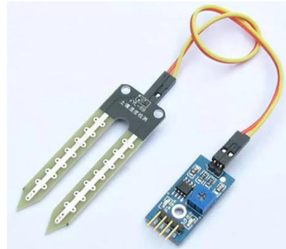
(b) The soil moisture sensor. 2
