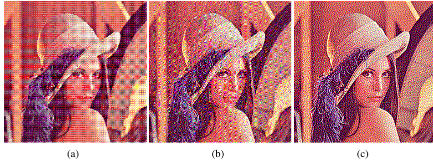
Fig. 1. The ordered dithering halftone image (a), Floyd and Jarvis error diffusion halftone images (b) and (c) generated from the color Lena image with the filters in Eq. (1) respectively
