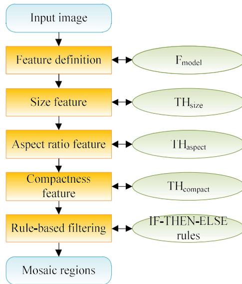
Fig. 6. Overall flow of the candidate filtering process.
