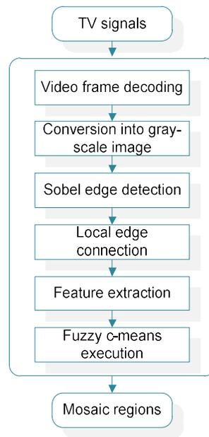
**Fig. 3.** Overall flowchart of the clustering-based method.
