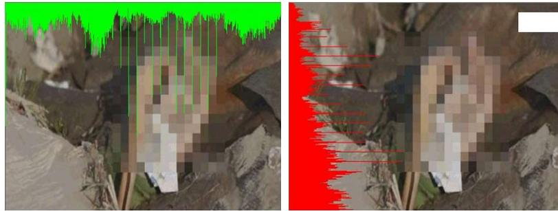
(a) Histogram of horizontally projected edges (b) Histogram of vertically projected edges
