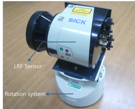
Fig. 1. A LRF sensor is mounted on a rotation base to construct the 3D laser scanner system.
