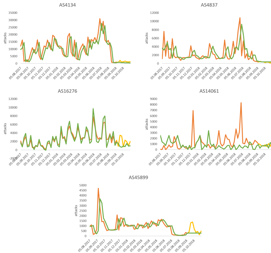
Fig. 4. An overview of MAPE results for predicting the number of attacks from individual autonomous systems. The green plot represents the real progression of attacks over time, with the orange representing the teaching run and the yellow in the foreground representing the model.
