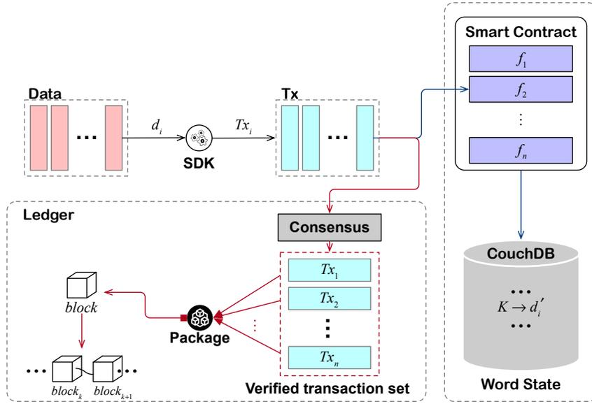
Fig. 1. Structure of the ledger in Hyperledger Fabric
