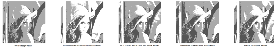
Fig. 5. Segmentation of the original gray image into three clusters using original image pixels intensities, from left to right via hard thresholding, multi-level thresholding, fuzzy c-means, subtractive clustering and kmeans clustering
