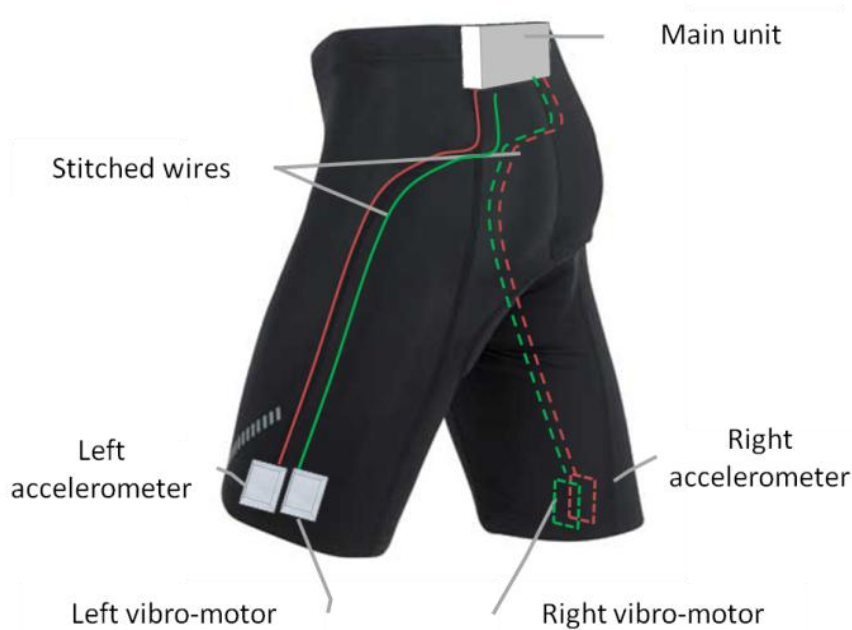
Fig. 2. The wearable rumble device mounted on spandex shorts
