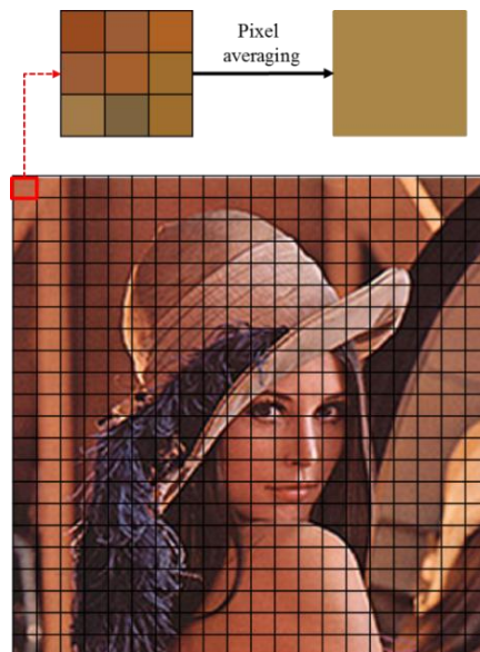
Fig. 7. Creation of virtual comparison blocks and pixel averaging
