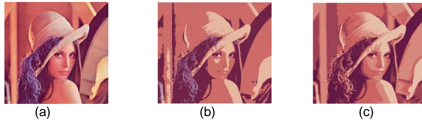
Fig.7. Segmented results of standard Lena image by the two algorithms. (a) Lena image template. (b) K-means (c) G-K-means.
