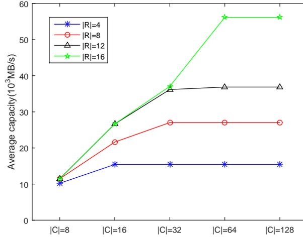
**Fig. 7.** Average capacity with  $C \times R = \{8, 16, 32, 64, 128\} \times \{4, 8, 12, 16\}$ .
