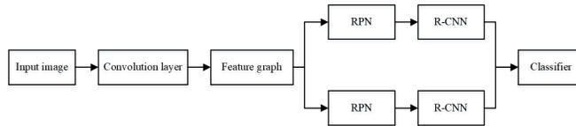
**Fig. 1.** Proposed network structure diagram of gesture recognition
