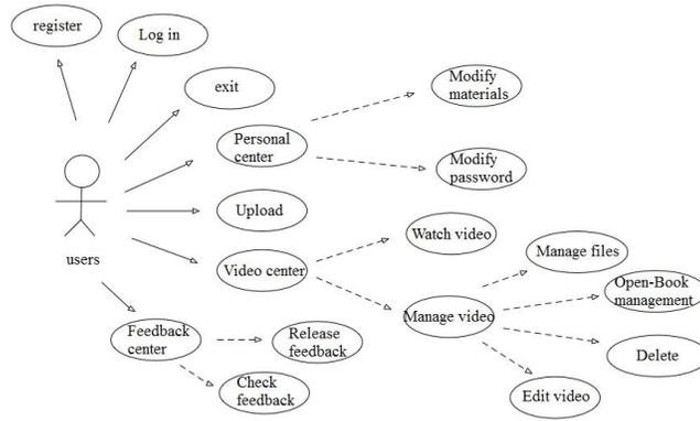
**Fig. 2.** Video Website Subsystem Use Case Diagram
