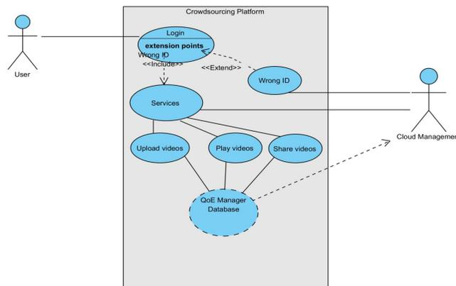
**Fig. 16.** Use Case Diagram of Crowdsourcing Platform
