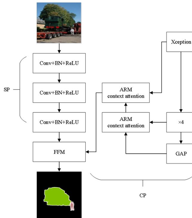
**Fig. 2.** Overall structure of proposed network model
