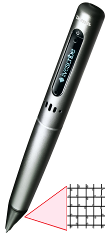
Fig. 3. Livescribe Smartpen and the dotted position system
