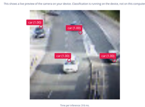
Fig. 7. Object detection from Arduino camera shown in browser
