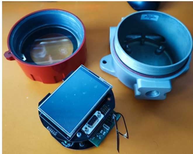
Fig. 1. Developed IoT node before sealing in the safety Ex e casing
