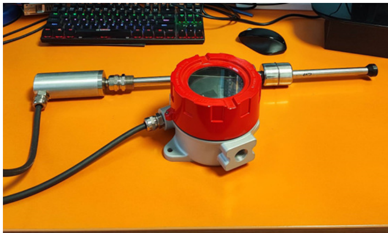
Fig. 11. Finalized IoT node with one RS485-based sensor attached
