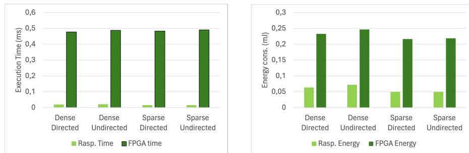
Fig. 9. Dijkstra: Avg. Time and Energy consumption within FPGA and Raspberry Pi
