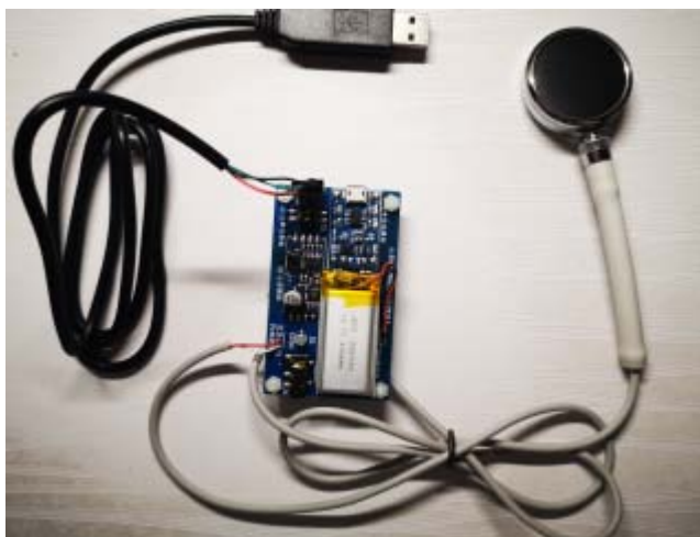
Fig. 3. Acquisition module of heart sounds
