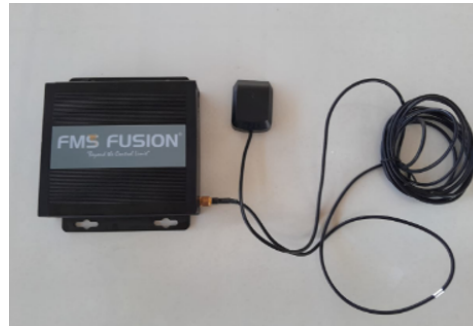
Fig. 4. The FMS Fusion device for collecting data
