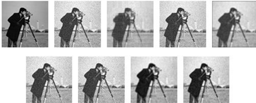
Fig. 3. Visual comparison of different denoising methods on the Cameraman with Gaussian noise (variance is 0.2). From left to right and top to bottom, the images are the Original image, Noisy image, and the denoised images obtained by RPCA, WSNM, Mean filter, Median filter, Bilateral filter, LPNF-PCA, and LPNF-LPP, respectively
