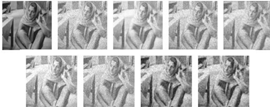
Fig. 4. Visual comparison of different denoising methods on the Barbara with mixed noise. From left to right and top to bottom, the images are the Original image, Noisy image, and the denoised images obtained by RPCA, WSNM, Mean filter, Median filter, Bilateral filter, LPNF-PCA, and LPNF-LPP, respectively
